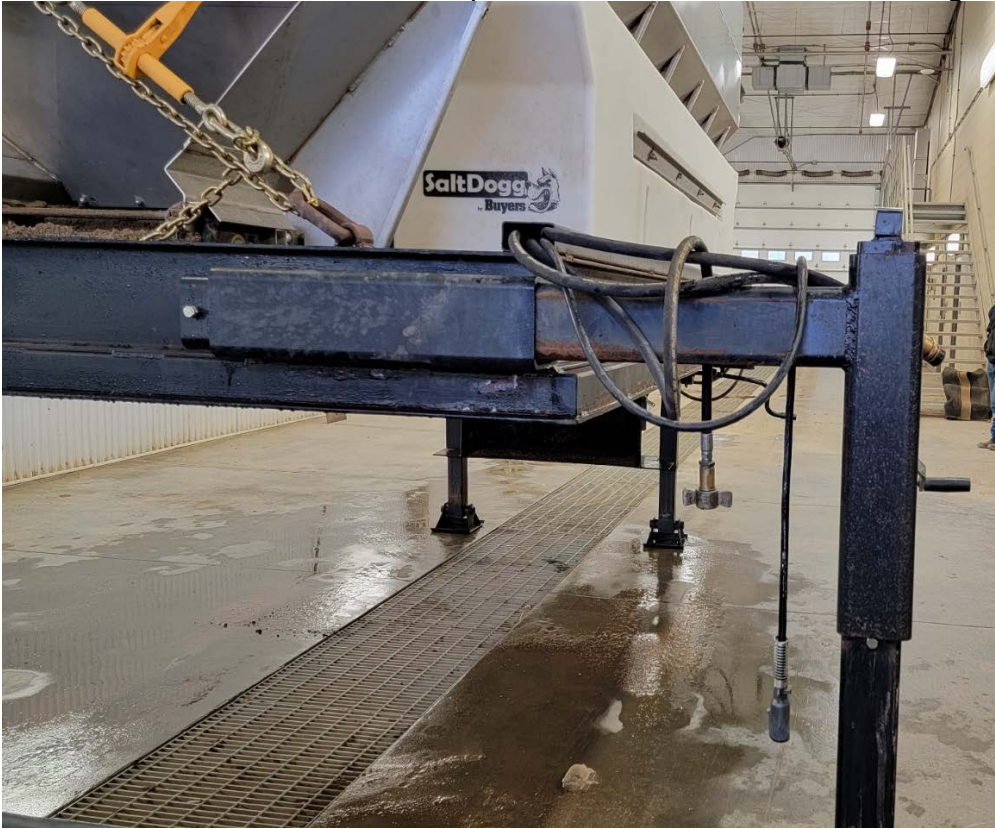
When not in use, the fifth-wheel quick-attach sander is free standing.
