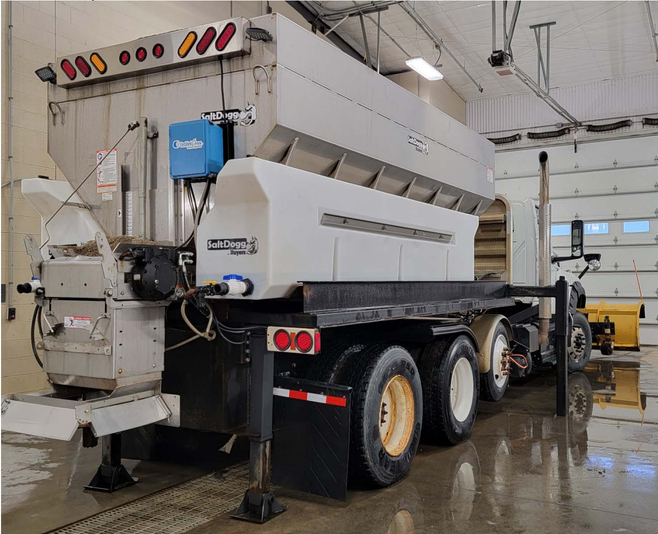
Fifth-wheel quick-attach sander on semi-tractor.
