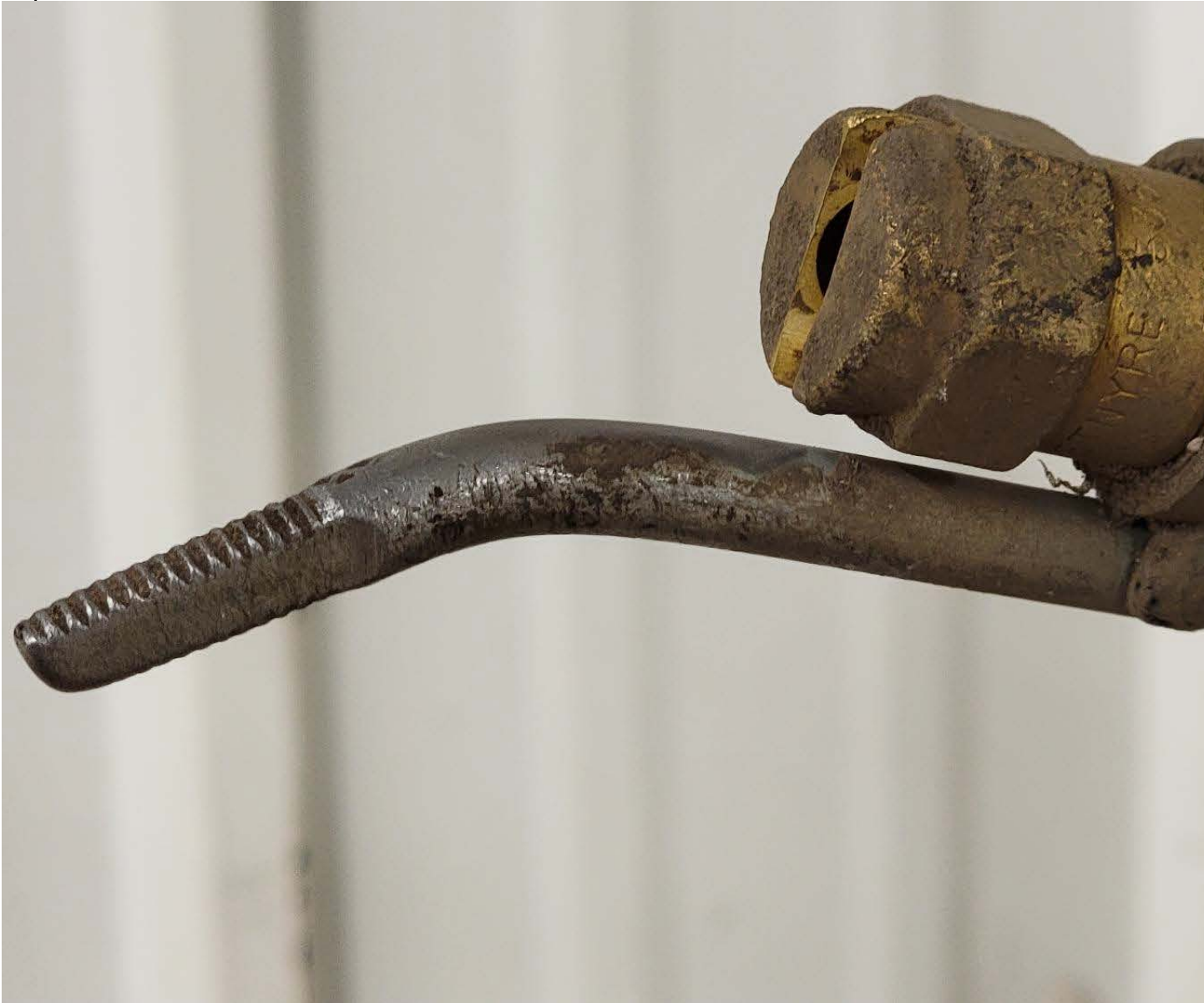
Asphalt Crevice Blaster
