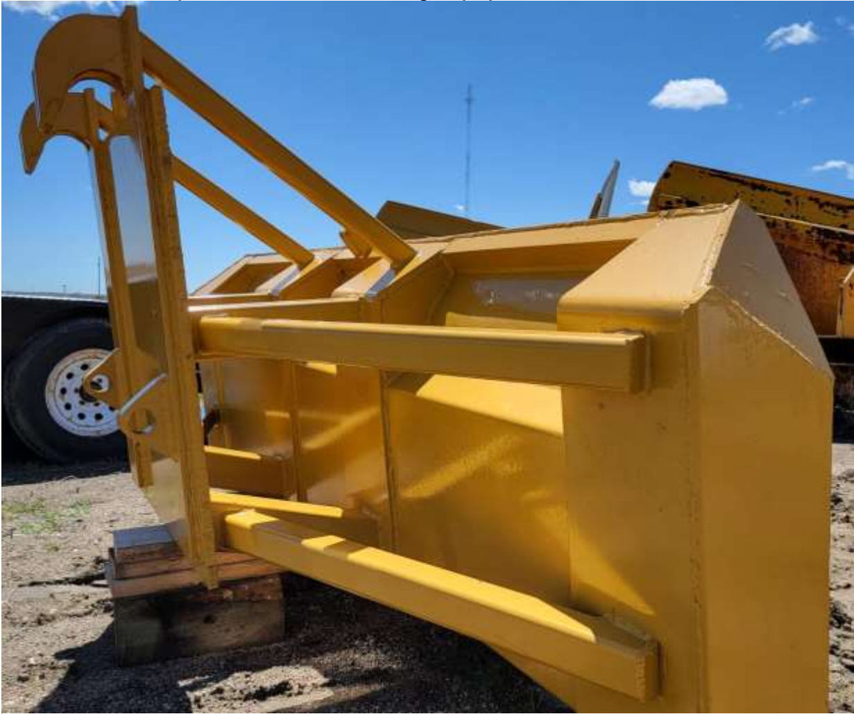
Side, backside of push-all dozer/ Falls lift group/quick attach hooks
