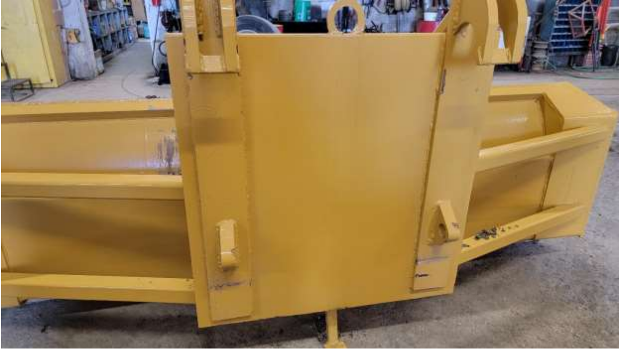
Steel push plate – falls quick attach group/hooks
