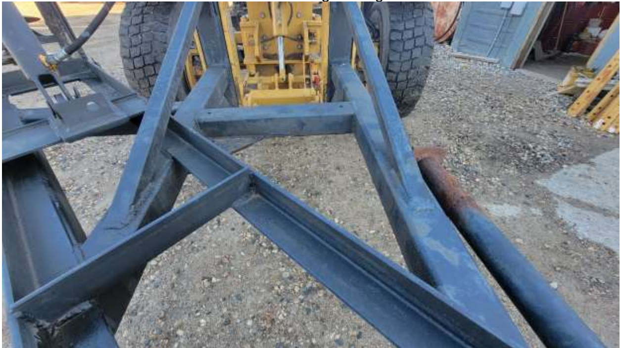
Disc base frame sets on Main frame at 45 degree angle.
