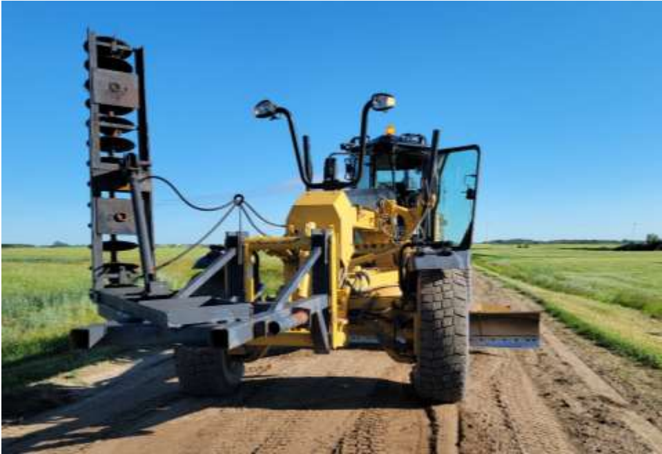
Hydraulic side disc in transport mode
