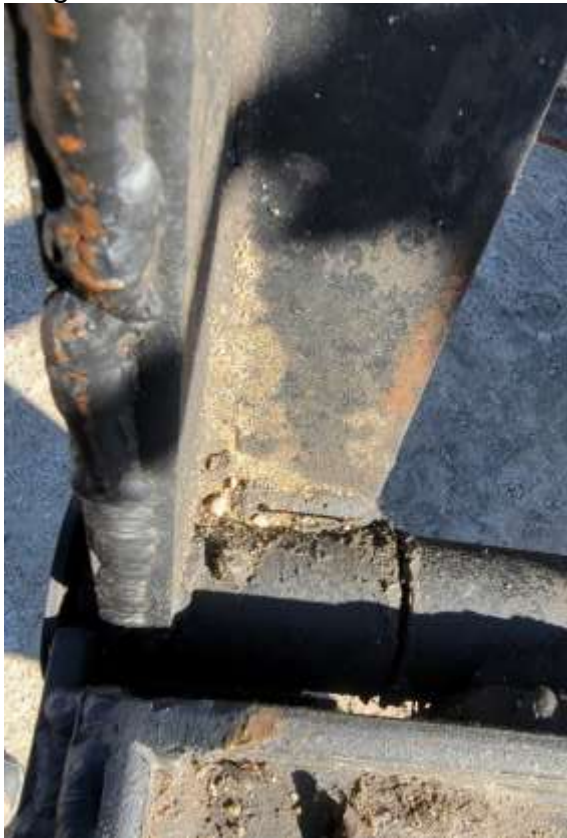
Hinge allows disc frame arm to flex
