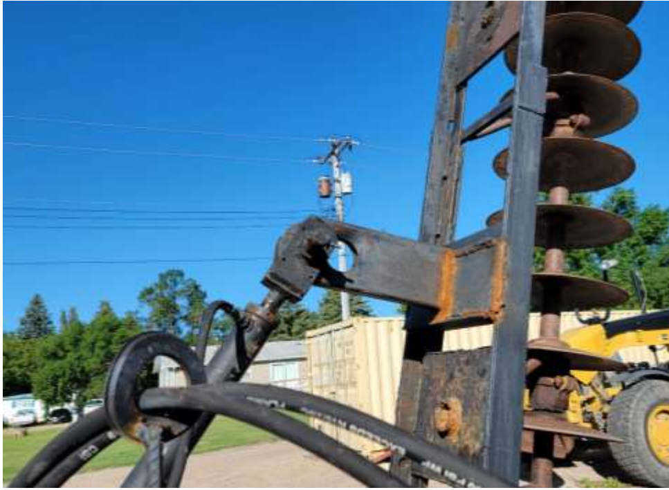
Hinge allows disc frame arm to flex
