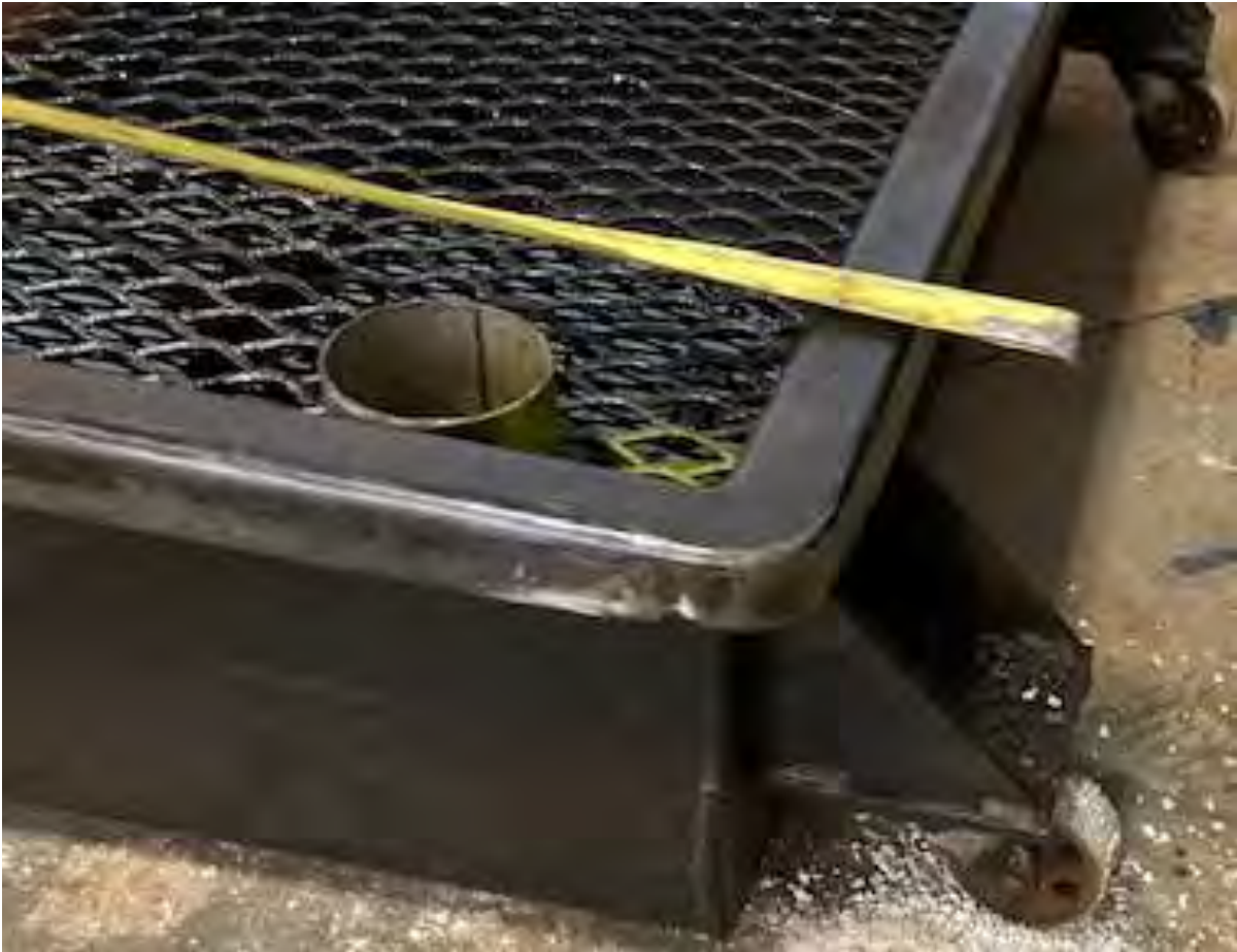
Trailer with collector screen, corner pipe for collection pipe, caster wheels
