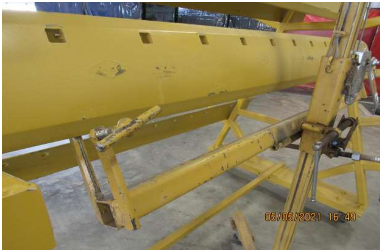
Only one person needed to remove cutting edge from rack (onto lift) then over to maintainer.
