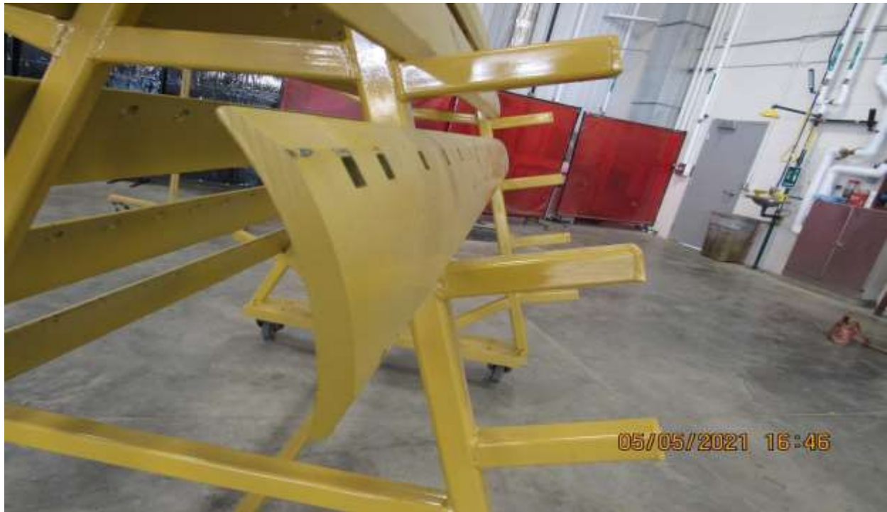
Only one person needed to remove cutting edge from rack (onto lift) then over to maintainer.
