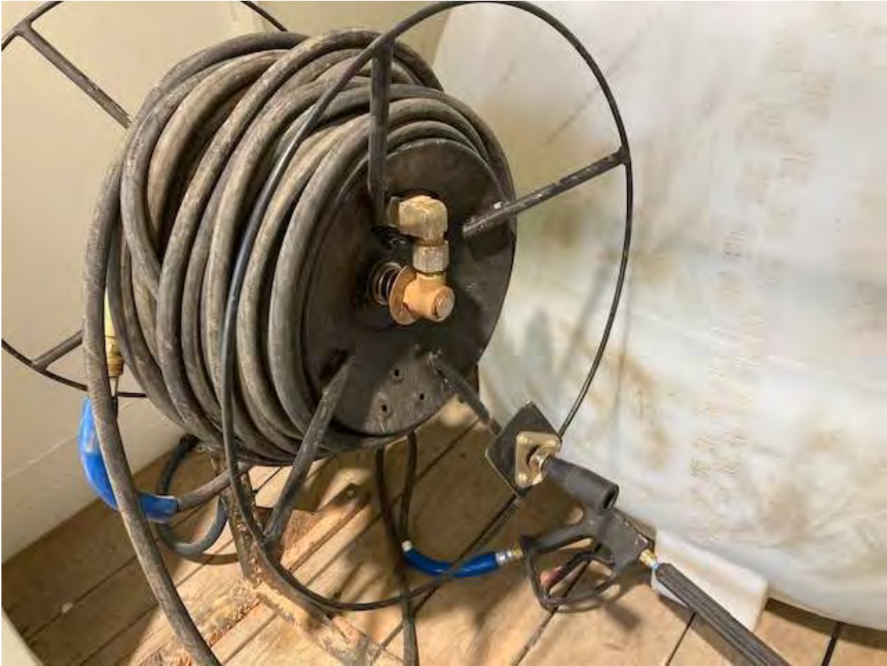
Hose reel with hose. Blue hose extensions connects the hoses, and the steamer to the reel.
