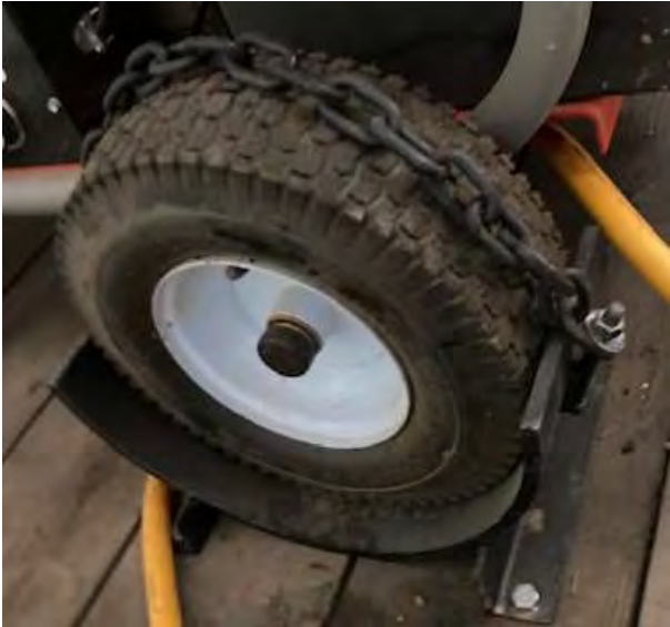
Power washer/water heater unit tie down
