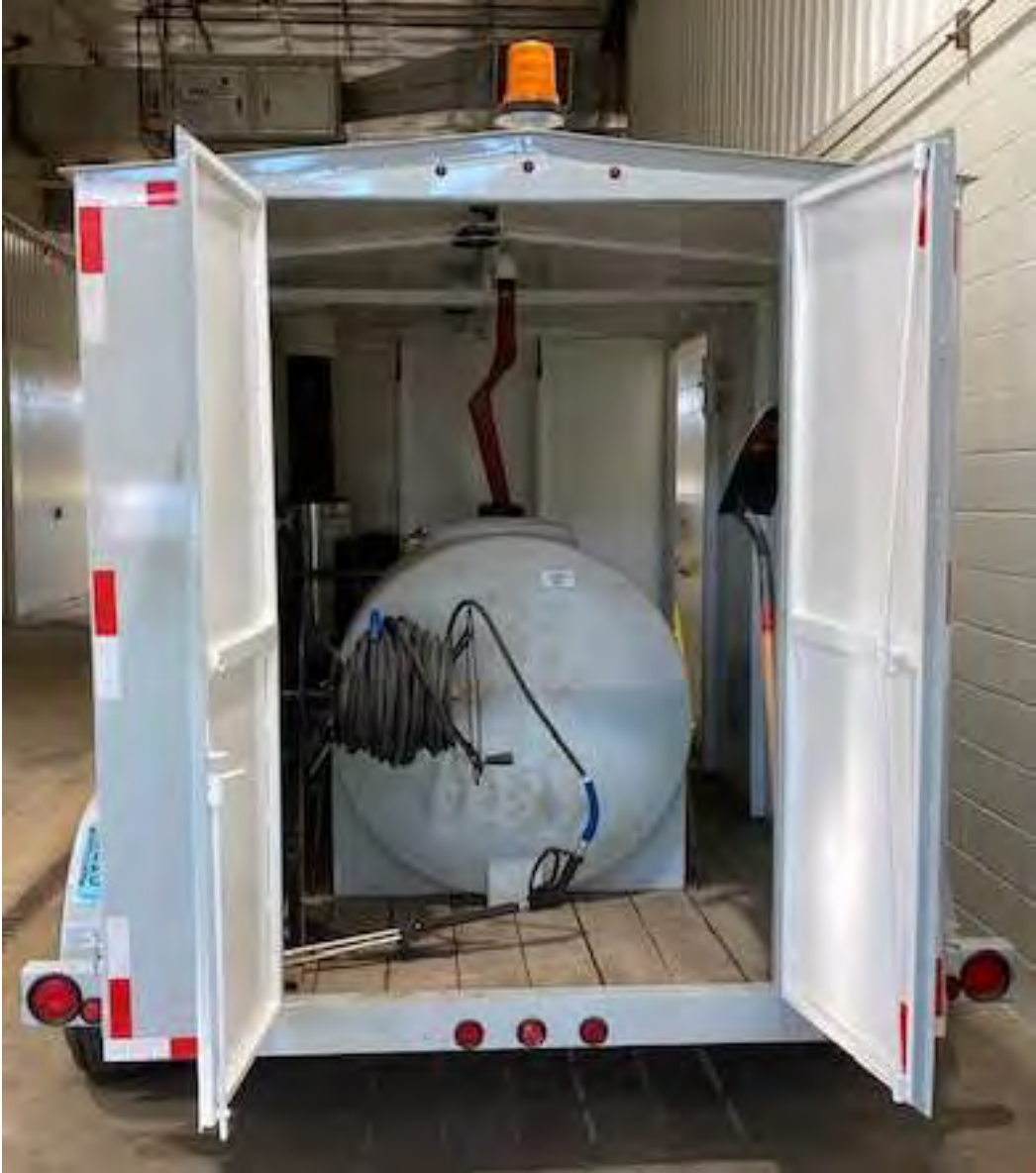
Interior of culvert steamer - water holding tank
