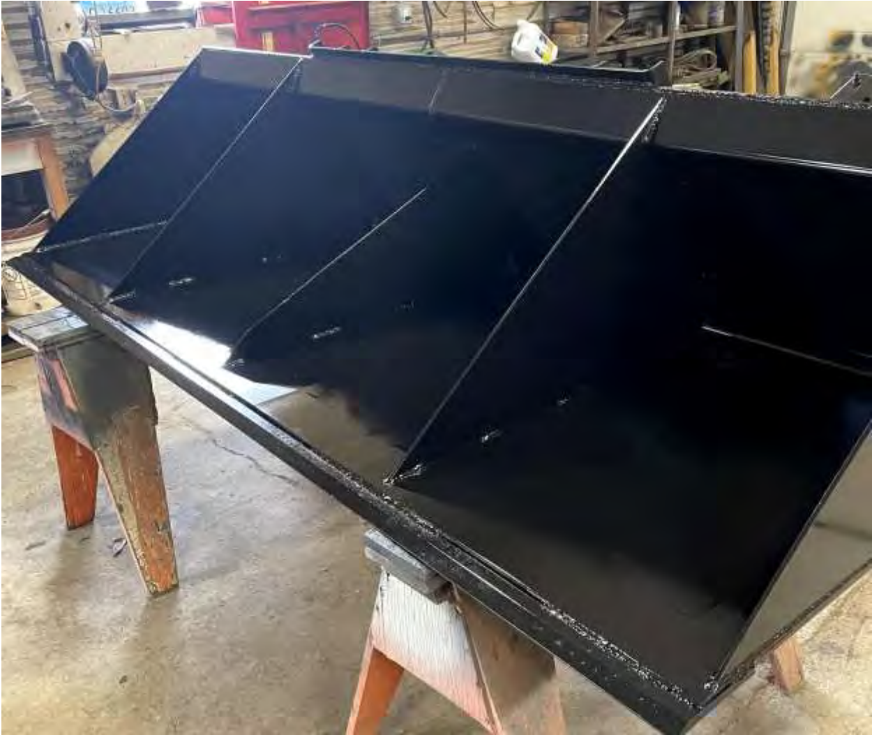
Front view, 3 feet deep, 8 feet wide Cutting edge welded bottom of bucket front
