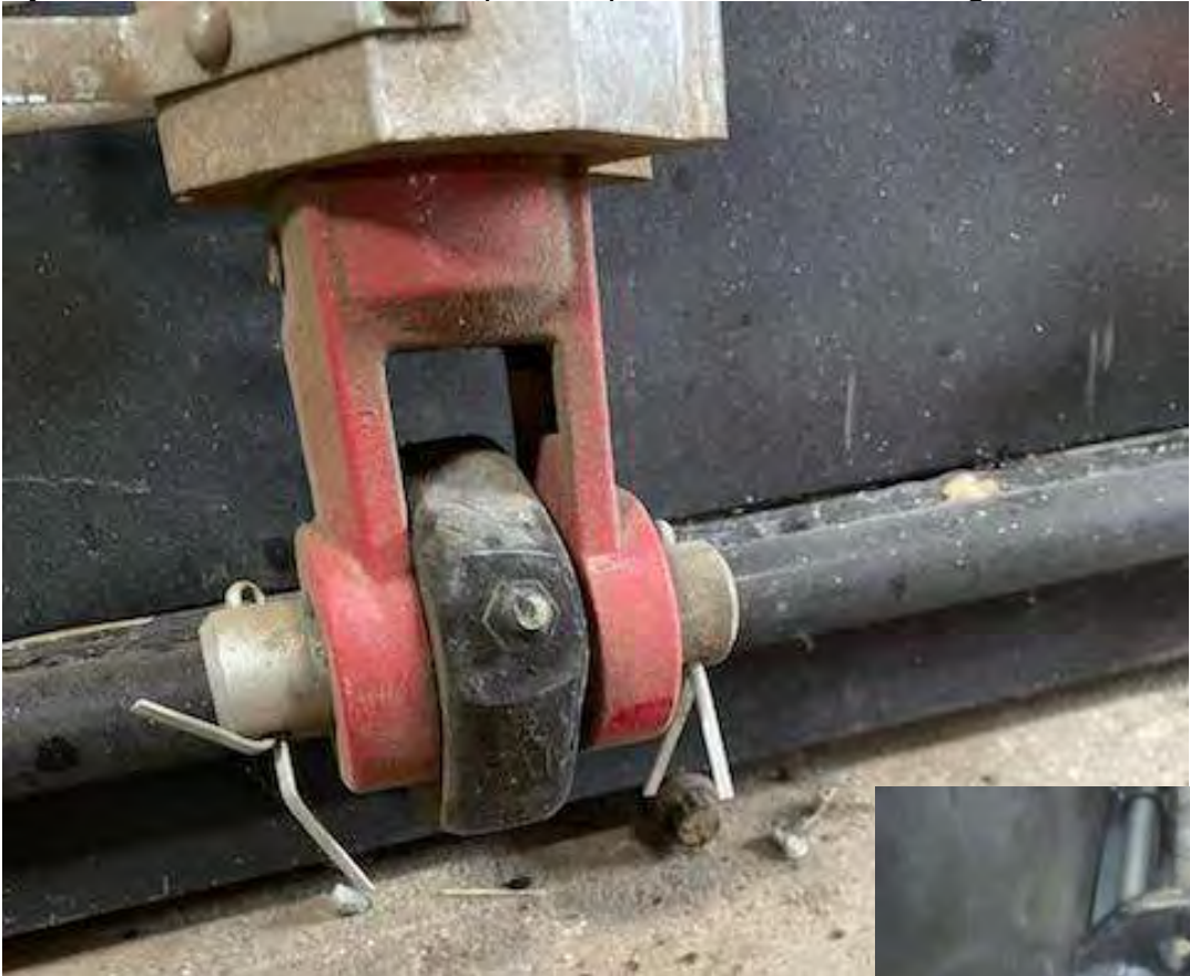
Cylinder attached to bracket, opens flap on bucket to release gravel
