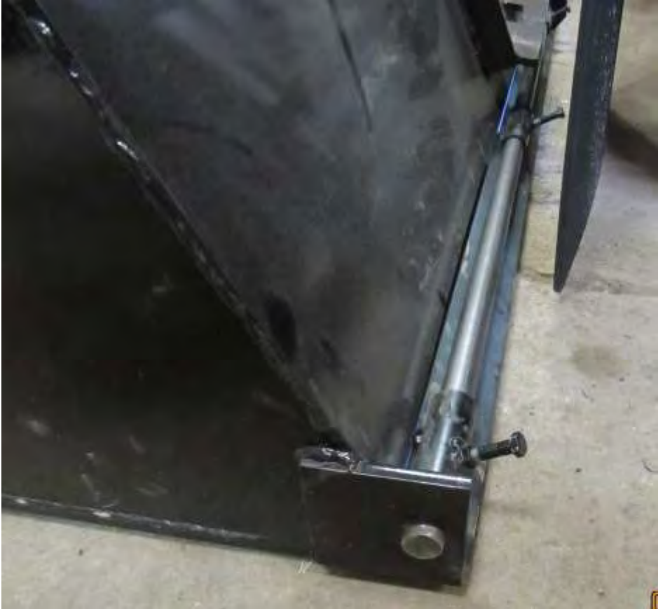
2x3" plates with 1" hole welded on each end of bucket, for 1" round shaft Hinges for flap door
