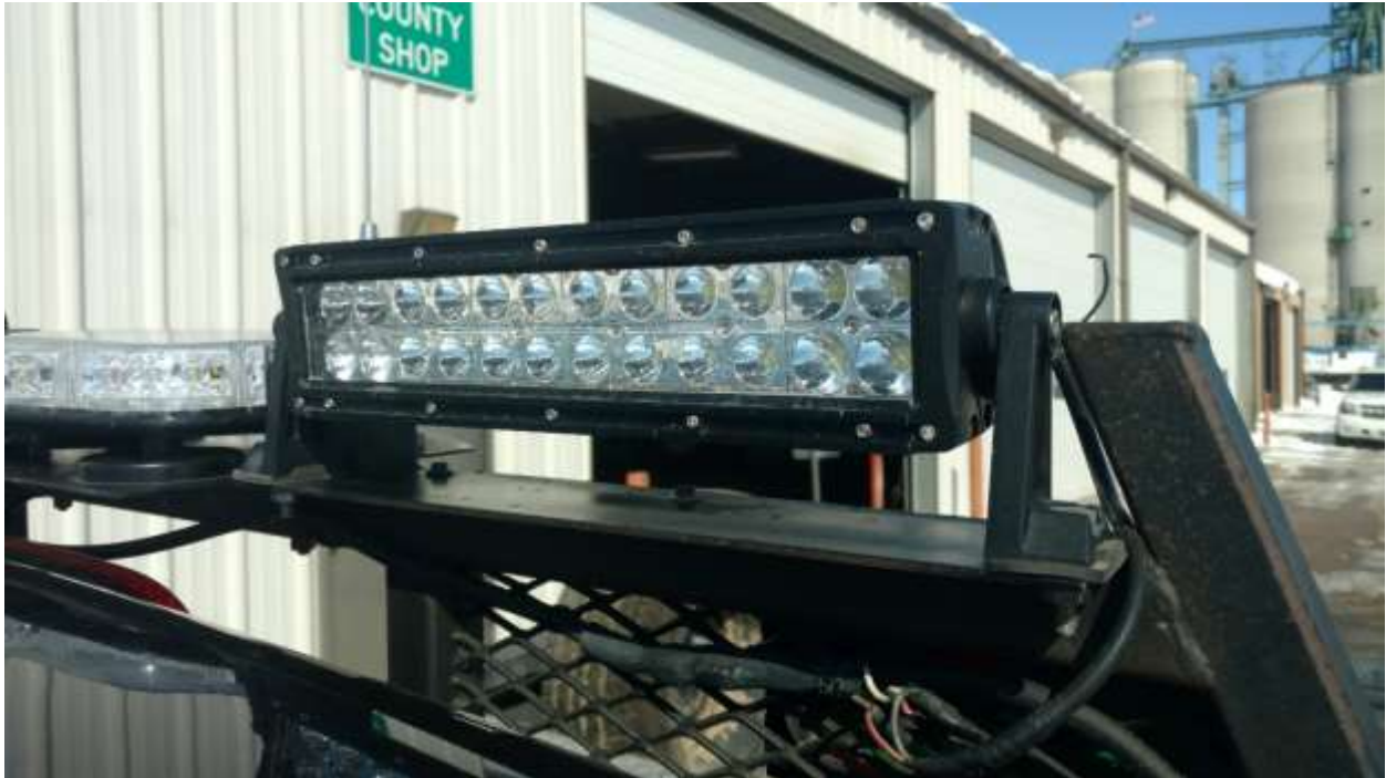
LED lights turned on to test sign reflectivity.
