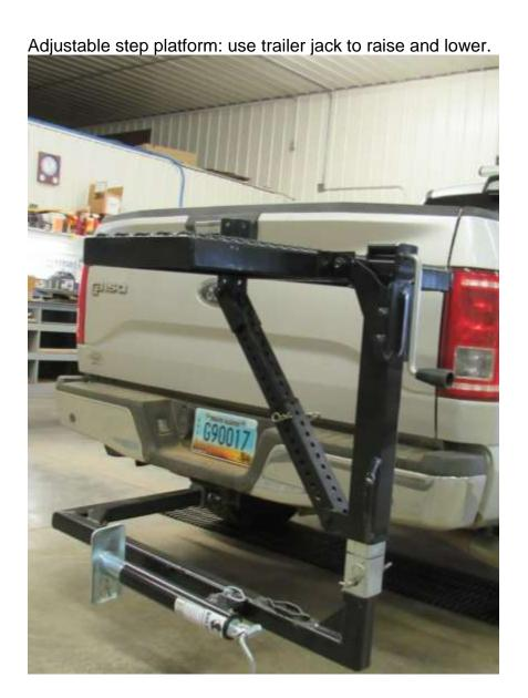
Adjustable step for ditch slope.
