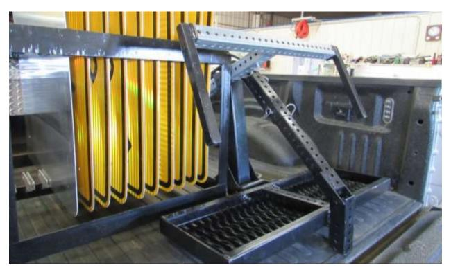
Sign rack – roads signs are easily accessible. No need to climb into pickup box to search through a multitude of signs laying on the bed.
