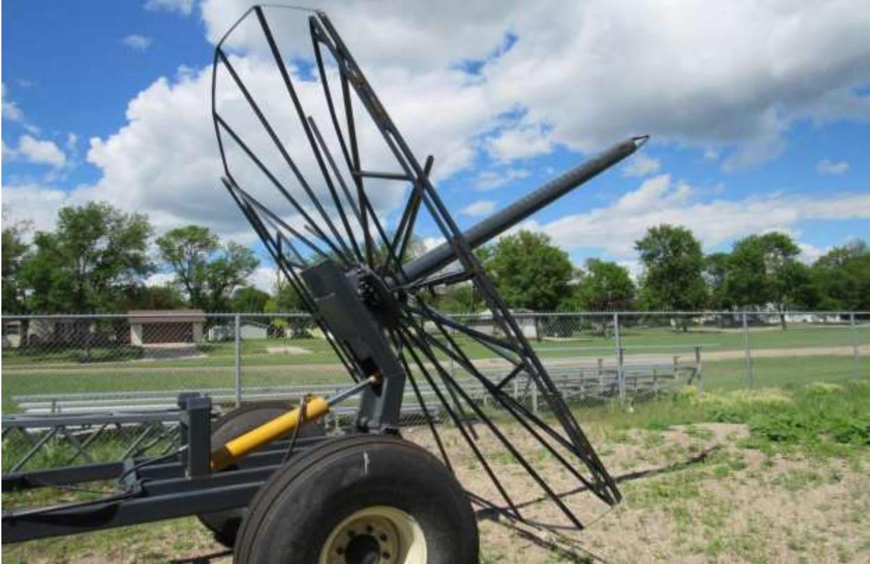
Hydraulic pump lifts spoke wheel bed.
