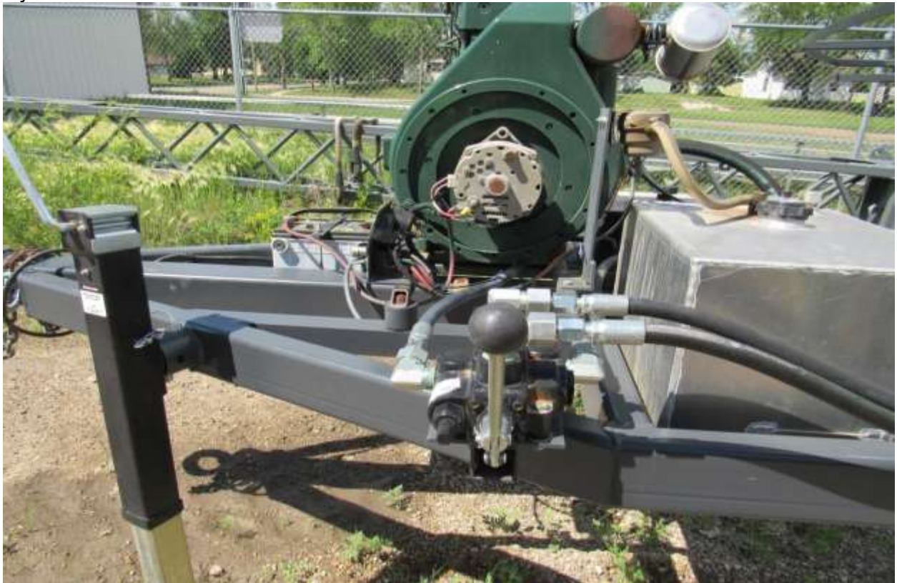
Safety bracket locks wheel to frame during transport.
