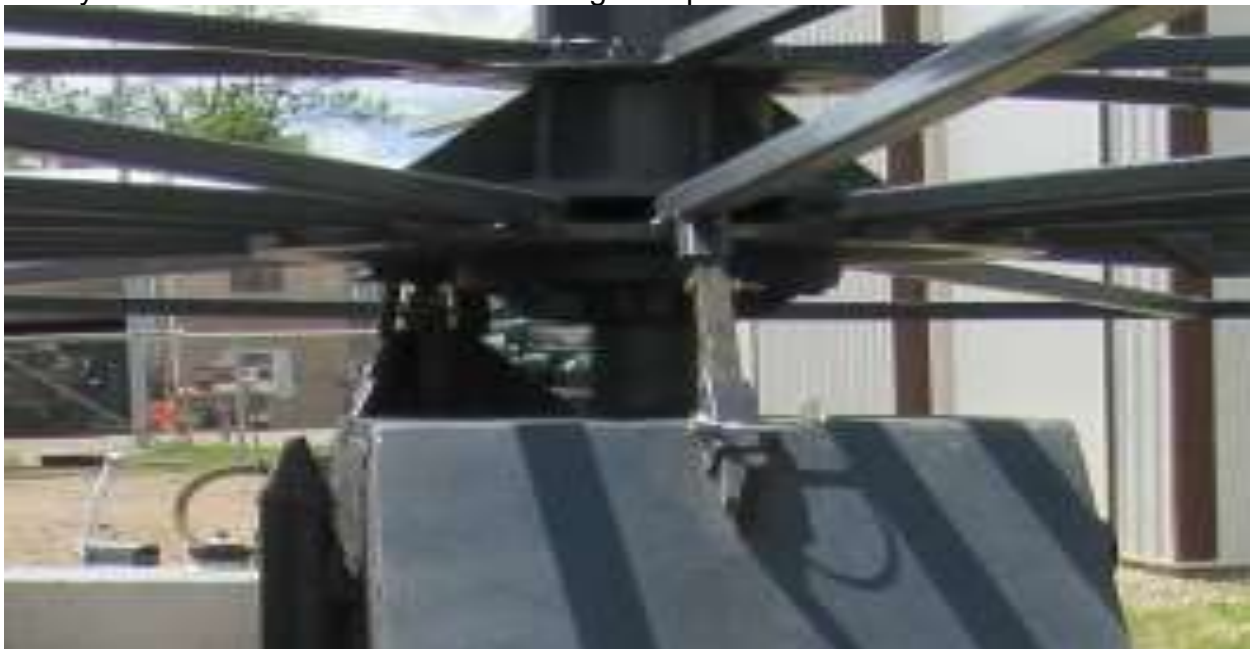
Safety bracket locks wheel to frame during transport.
