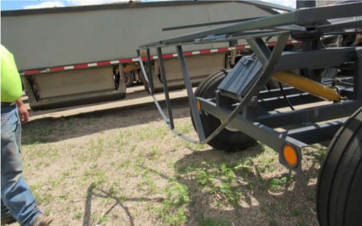
Rear of spoked wheel folded down prior to lifting bed.
