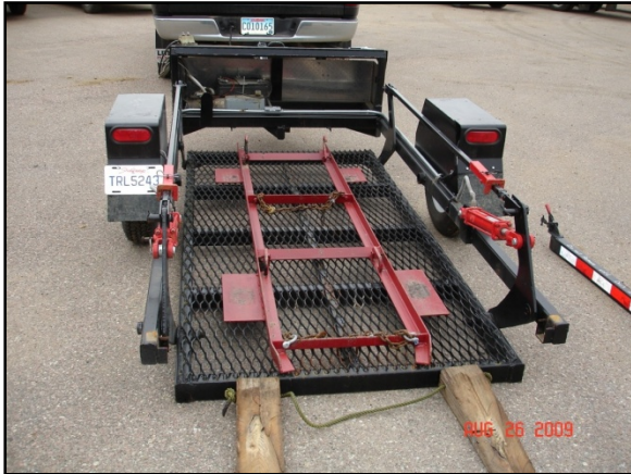
Trailer with deck dropped to ground
