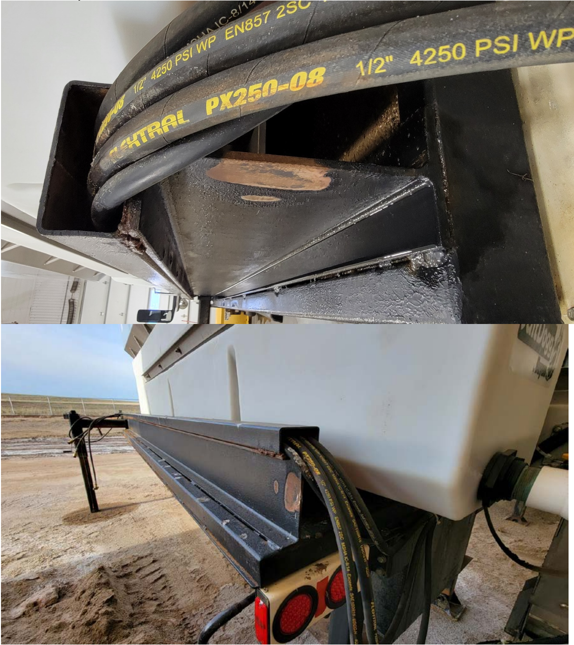
Conduit to protect hoses.
