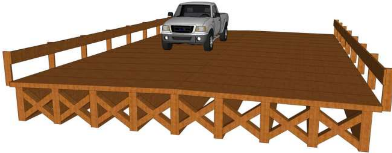
50-ft long, 34.5-ft Wide Girder Bridge
