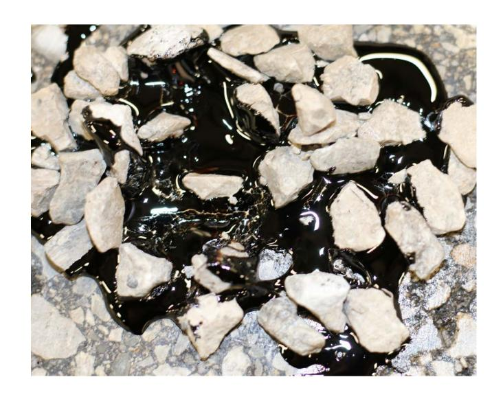
Wet Aggregate and Surface with Cutback prevents good adhesion MC-3000 is prevented from bonding to the surface if the pavement or aggregate is wet
